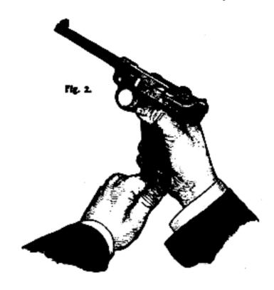
in illustration 2, the thumb of the right hand can press the catch (27); simultaneously the cartridge holder is either withdrawn with the left hand by the bottom piece, or, in case of urgency, simply allowed to drop out so that the left hand can insert another one immediately.
